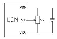
$V_{\mathrm{DD}} \sim V_0$ : LCD Driving voltage
